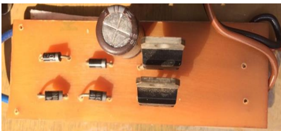
Fig.7.Connection of power supply on PCB
